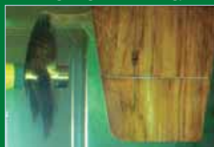
TLKSR® cavitation test – no cavitation
