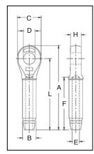
NOTE: S-502 Swage Sockets are recommended for use with 6 x 19 or 6 x 37, IPS or XIP (EIP), XXIP (EEIP), RRL, FC or IWRC wire rope. Before using any National Swage fitting with any other type lay, construction or grade of wire rope, it is recommended that the termination be destructive tested and documented to prove the adequacy of the assembly to be manufactured.
