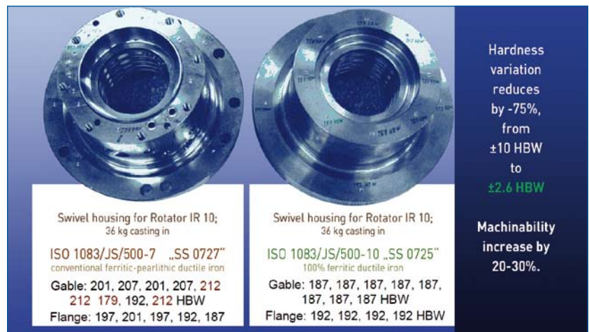
Fig. 3: Swivel housing: Distribution of the Brinell hardness over the cross-section of the casting when GJS-500-7 or GJS-500-10 is used [6/
