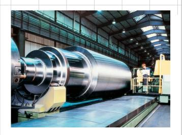
Customer demand for increasingly wide plates required correspondingly wide rolling mills. GP met these demands in its own roll production with expanded dimensions and increased weights of up to 265 tons per piece.
