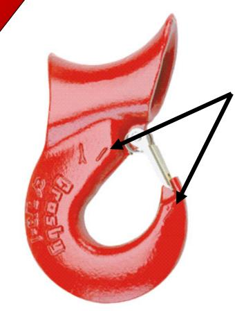
Deformation Indicators -- Two strategically placed marks, one just below the eye and the other on the hook up, which allows for a QUIC-CHECK® measurement to determine if the throat opening has changed, thus indicating abuse or overload.
