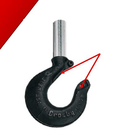
**Deformation Indicators** -- Two strategically placed marks, one just below the shank or eye and the other on the hook up, which allows for a **QUIC-CHECK**<sup>®</sup> measurement to determine if the throat opening has changed, thus indicating abuse or overload.
