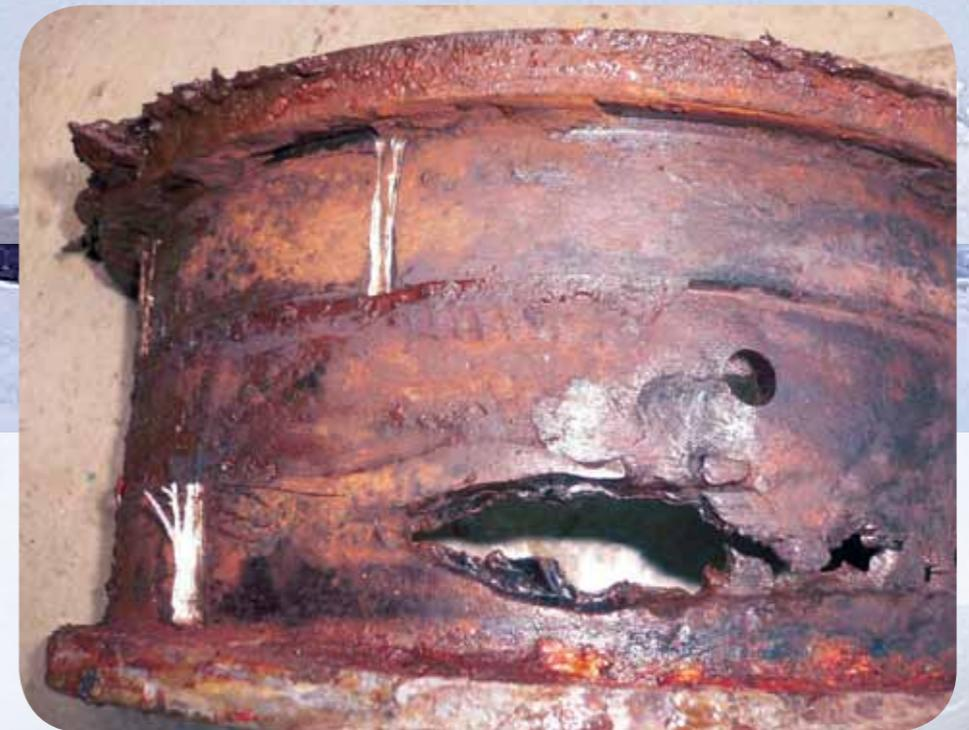
A painted grease nipple can cause damage to a non-lubricated bushing.
