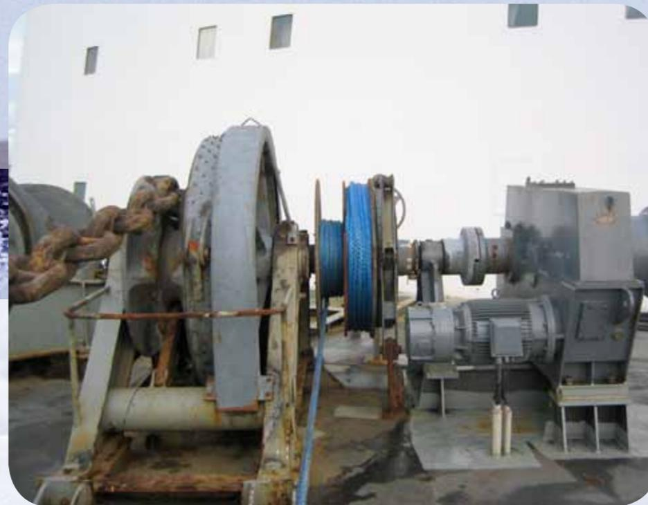
HATLAPA's advanced frequency controlled electric drive system replaces maintenance-intensive electro/hydraulic drives
