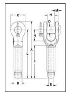
NOTE: S-501 Swage Sockets are recommended for use with 6 x 19 or 6 x 37, IPS or XIP (EIP), XXIP (EEIP), RRL, FC or IWRC wire rope. Before using any National Swage fitting with any other type lay, construction or grade of wire rope, it is recommended that the termination be destructive tested and documented to prove the adequacy of the assembly to be manufactured. In accordance with ANSI B30.9, all slings terminated with swage sockets shall be proof loaded.\*
